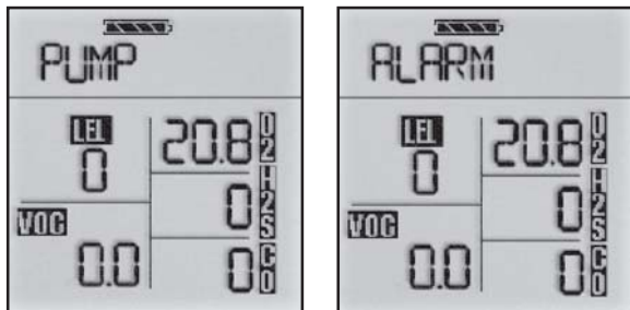
Figure 6: PUMP/ALARM flashing on the display
