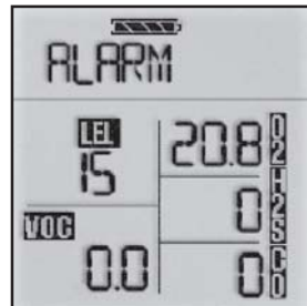
Figure 8: Instrument in LEL Alarm
