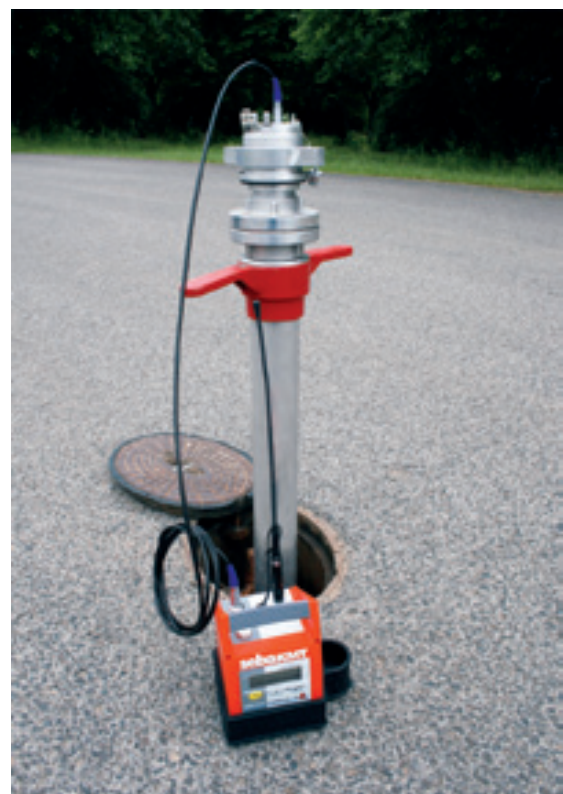
PAM HYDRO-2 connected to a P-2 correlator transmitter
