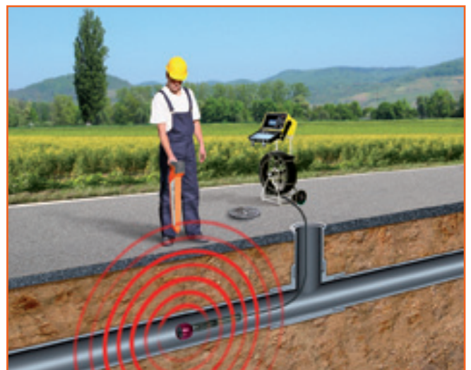
Location of Sewer TV Camera with Easyloc Cam
